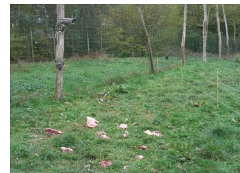
Fig. 3. Meat left during an experiment in the grey wolf enclosure. In this case, a two-wire fence was tested. A thermal camera and two remote cameras can be seen, fixed on wooden poles and facing towards the fence or meat.
